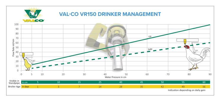
of the drinking lines as well as the pressure in the lines should 'grow', and the chickens grow the fastest in the first two weeks. The above graph recommends water pressure in the watering system corresponding to the bird age with related water flow.
