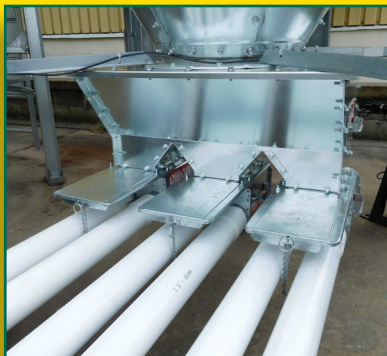
The Triple Upper Boot is designed to provide more feed to more flexible auger lines from one source. When used in conjunction with the double lower boot, up to six auger lines can run from a single feed bin!
