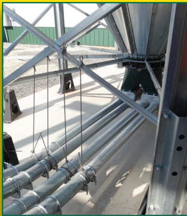
A double boot, twin transition application for maximum versatility and delivery rate.
